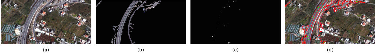
Figure 5: Figures 5a, 5b, 5c and 5d show the original image, besides applying road detection, vehicle count, and the results fusion, respectively, for Study Area 2.
