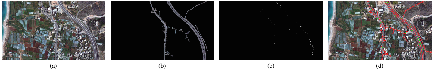
Figure 6: Figures 6a, 6b, 6c and 6d show the original image, besides applying road detection, vehicle count, and the results fusion respectively, on Study Area 3.
